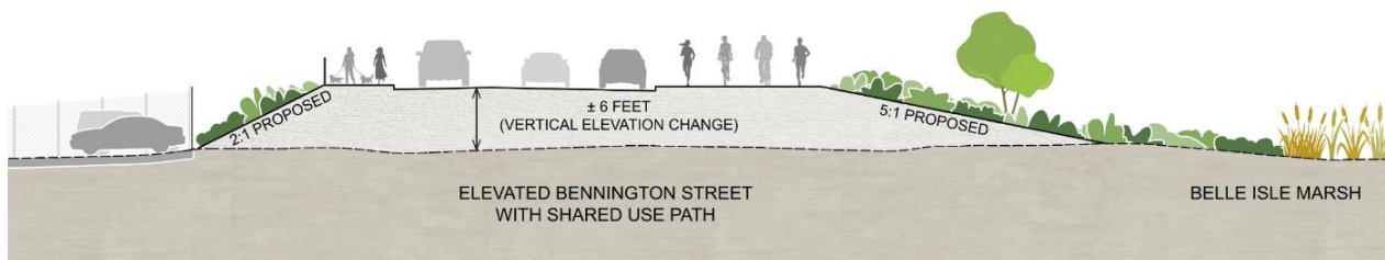
Figure 6: Alternative BS-1 Elevated Roadway—Illustrative Cross-Section (Terraink)
