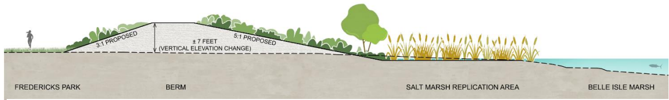
Figure 1.19: Living Levee with Salt Marsh Replication—Illustrative Cross Section (TerrainK)
